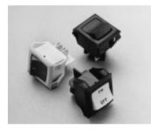
The RGSC-Series Super Curvette rocker switches offer the Curvette styling in a double pole construction with higher electrical ratings and high inrush capabilities. These switches can handle up to 125 amp peak inrush current and can accommodate a wide range of panel cutouts due to the patented mounting ear construction. International ratings are available up to 20 amps.
